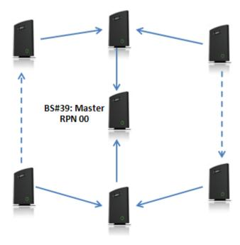
Depending on the system setup, it is recommended to place the Sync source Master in the middle of the building and to assign numbers/addresses, radio ID (RPN), etc. to each base station or repeater for easy identification.
