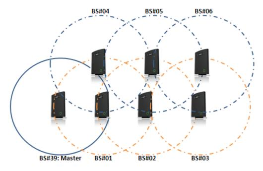
BS#39 is the SYNC Master, if BS#05 is down, most user handovers can be formed via 3 other alternative cells (i.e. BS#06, BS#02 and BS#04), but cannot operate in the coverage area of BS#05 where no other base station can reach the handset.
