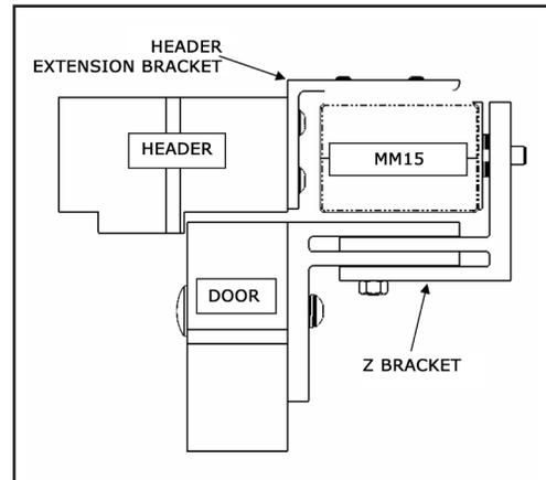
**2.** Place a 1/4" spacer on the Z-Bracket and then place the MM15 on top of that with the armature engaged with the MM15.
