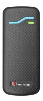
The SIFER card reader is a Smart Card reader designed and manufactured by Inner Range. It is a multi-drop RS-485 based reader that employs 128 bit AES encryption from the card through to the door module, providing a far superior level of security than that of traditional Wiegand based card readers. SIFER readers utilise the Mifare DESfire EV1 card format.
