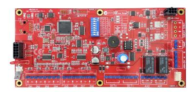
The 8 Zone LAN Expander Module also offers a UniBus in-cabinet expansion interface allowing further expansion of Zone inputs and Auxiliary outputs using plug on UniBus expansion devices fitted within the same tamper protected enclosure. Up to 32 Zone Inputs or 32 Auxiliary Outputs can be connected to the Module (32 Zones and 26 Auxiliaries or 24 Zones and 32 Auxiliaries at the same time).
