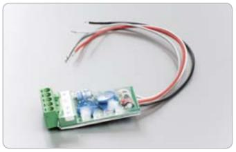
Where Concept 4000 hardware is installed in locations and environments where a very high level of electrical transient activity might be anticipated, the addition of Inner Range Advanced Surge Protection Devices adds a further layer of transient protection.
