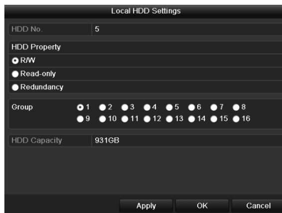
Figure 13. 13 Local HDD Settings Interface
