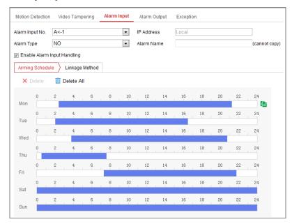
Figure 9-8 Alarm Input Settings
