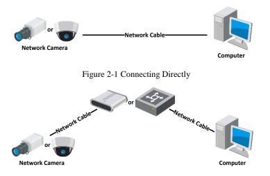
Figure 2-2 Connecting via a Switch or a Router
