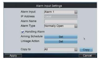
(5) Set the handling action for the selected alarm input by clicking the checkbox of Handling Alarm.
