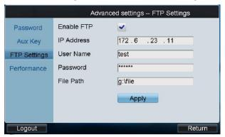
2. Check the checkbox of Enable FTP.
