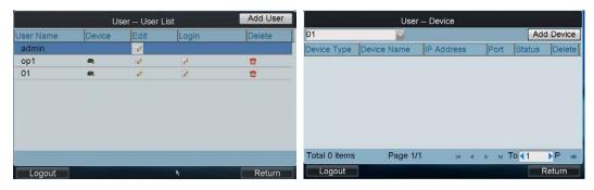
Click Add Device to enter the User-Add Device interface. Select the device by clicking the checkbox, and click Add to add the device for the current user.
