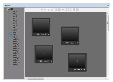
The corresponding output channel is corresponding to the Index No. on the Screen Group interface of the keyboard, e.g., the index 1 corresponds to the 108\_vga\_0 output channel.
