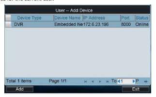
3. The successfully added device is listed on the **User-Device** interface.
