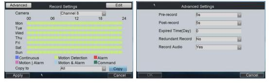
**Pre-record:** The time you set to record before the scheduled time or event. For example, when an alarm triggered the recording at 10:00, if you set the pre-record time as 5 seconds, the camera records it at 9:59:55.
