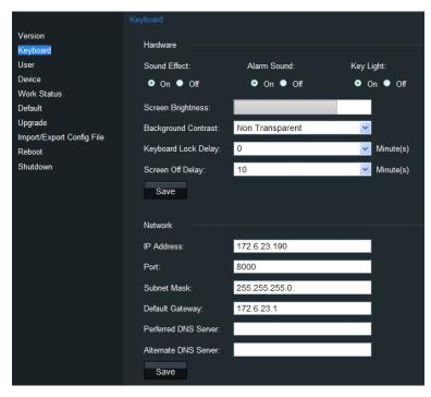
On this interface, you can configure the hardware and network parameters of the keyboard.
