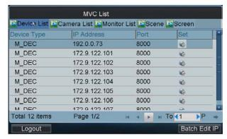
The device types in the MVC system are shown as follows:
