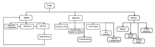
**Admin:** For the first time to operate the keyboard, you should configure the keyboard parameters in Keyboard Configuration menu, add device and operator, and then link the added device to assigned operator.
