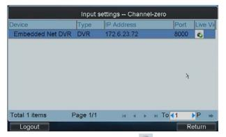
2. Select an encoding device from the list and click the icon to enter the local live view by the channel-zero.
