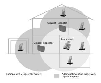
Before you start to register the units, install the Gigaset Repeater in close proximity to the base station and a power supply point. If a Gigaset Repeater is already in use, it must be switched on and positioned next to the base station before registration can commence.
