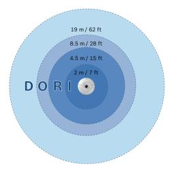
When mounted at a height of 3 m (10 ft) the 180° version of the camera has the following coverage radius for the four levels:
