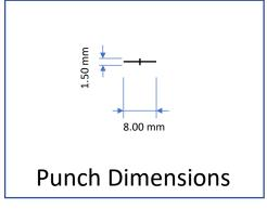
Punching a hole of the correct dimensions in the correct location will not impact on the SIFER cards warranty.
