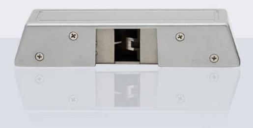
Lockwood Padde Series ES6000 Hook Lock is suitable for swinging doors, sliding doors and is easily attached to wood or steel door frames. ES6000 is heavy duty designed with its high preload (side load) capability of up to 300 kg, high holding force of up to 700 kg and up to 4hr fire rating. Both Power to Open and Power to Lock models are available.
