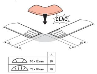
For mounting with floor ducts 92x20mm
