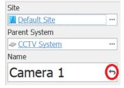
• Integrated Devices: When creating Integrated Devices with connections directly to the endpoint (Cameras, Intercom Points, etc) a parent Integrated System will be automatically created for the new device. This allows common settings, such as the event monitoring options, to be configured from a central point, rather than individually for all endpoints.
