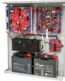
IAC Controller shown in 8 Door configuration.
