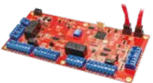
21220 UniBus 2 Door / 2 Reader expansion-board PCB
