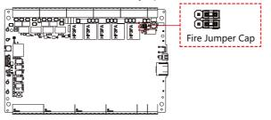
The position of the fire jumper cap position and the related NO/NC status are as follows:
