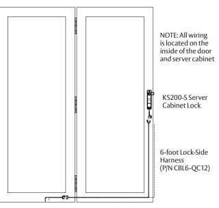
12-foot System-Side Door Harness (P/N CBL12-QC12) to EAC Panel Connection
