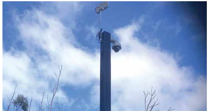
Remote power for bushfire monitoring cameras with IR and cloud communications in Victoria, Australia.
