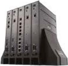
iPECS UCP is Ericsson-LG Enterprise's Internet Protocol (IP) and unified communications platform designed to meet the SMB and Enterprise communications needs. iPECS UCP uses advanced packet voice and IP switching technology, which is combined with UC&C, mobility solution and business applications.
