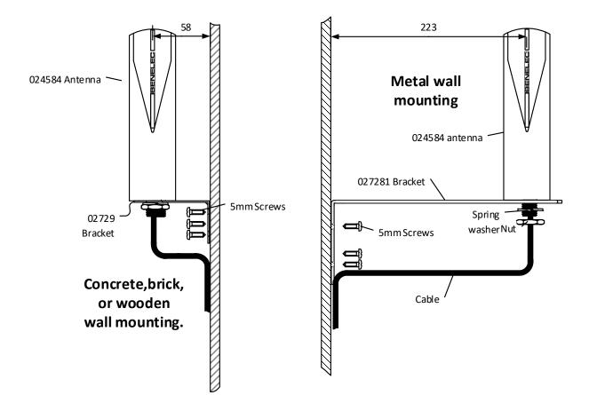
For wall mounting the 024584 antenna must be mounted according to the type of mounting surface material. Close mounting to metal surfaces will affect the VSWR and radiation pattern shape and performance. The use of the bracket 027281 is recommended when mounting against a metal surface.
